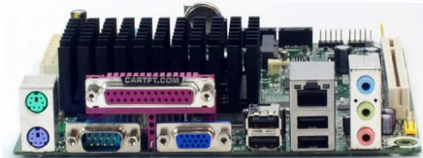
The Intel® Desktop Board D525MW is designed to unleash the power of the new Intel® Atom™ processor D525 which supports the new revolutionary two-chip layout. This new chipset layout reduces the package footprint by 70 percent, enabling easier routing and better heat flow. The Intel® NM10 Express Chipset also provides additional flexibility and upgradability with two slots of single channel DDR3 memory at 1066/800 MHz supporting up to 4GB maximum.
